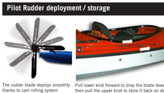
The rudder blade deploys smoothly thanks to cam rolling system Pull lower knot forward to drop the blade down, then pull the upper knot to store it back on deck.
