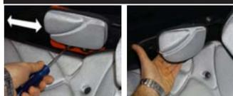
Slack mounting screws to adjust back and forth
