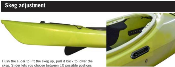
Push the slider to lift the skeg up, pull it back to lower the skeg. Slider lets you choose between 10 possible positions
